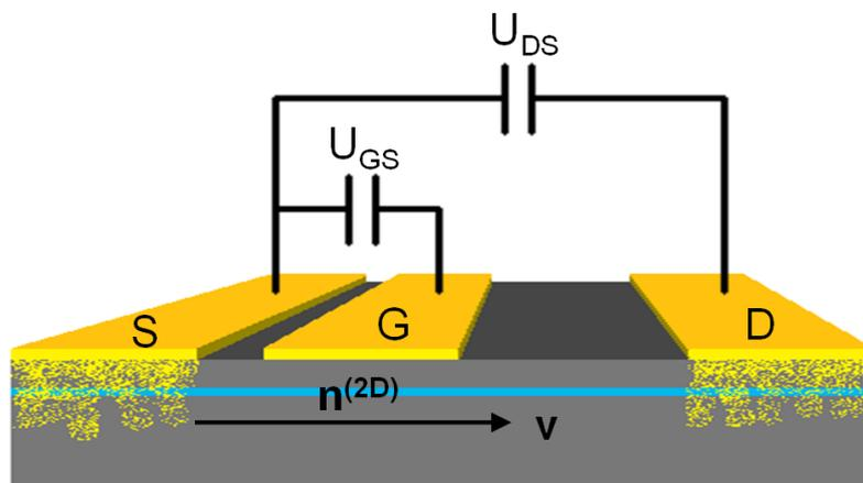
*Fig. 2: Schematic of a FET*
