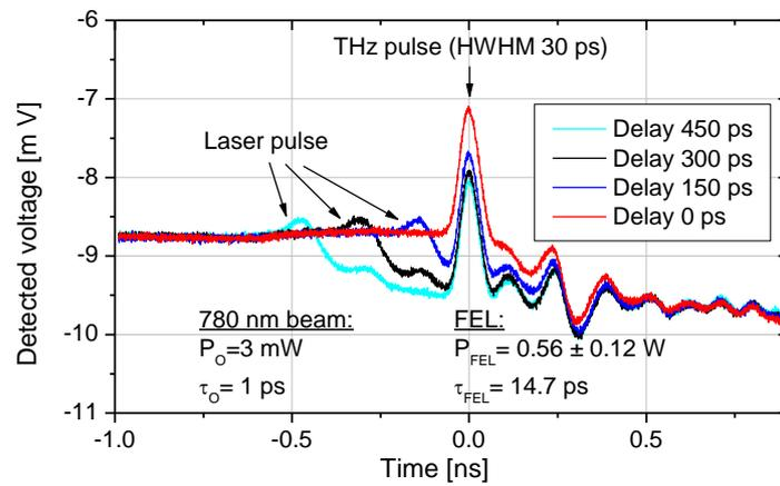
Fig. 4: Synchronous measurement of a free electron laser pulse and a NIR laser pulse with a LA-FET and a 30 GHz oscilloscope. [\[Link zum Paper\]](#)
