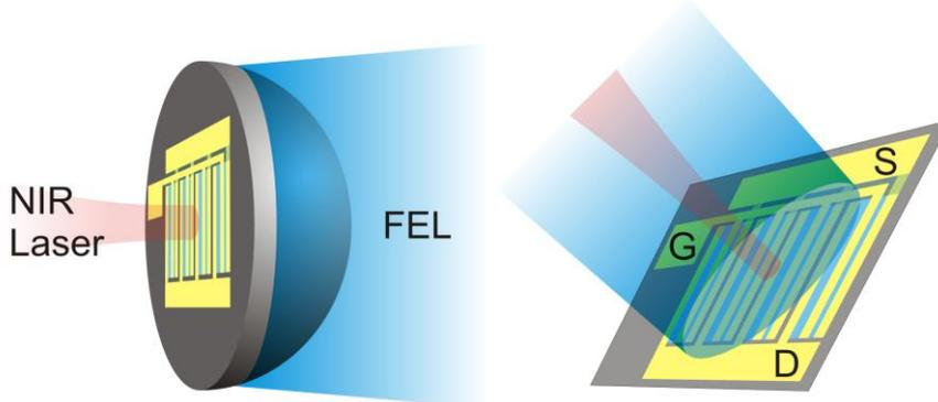
Fig. 3: Schematic layout of a LA-FET. Left: silicon-lens coupled device (typical cross section  $\sim 0.3 \times 0.3 \text{ mm}^2$ ). Right: free space device (typical dimensions  $\sim 1.2 \times 1.2 \text{ mm}^2$ ).
