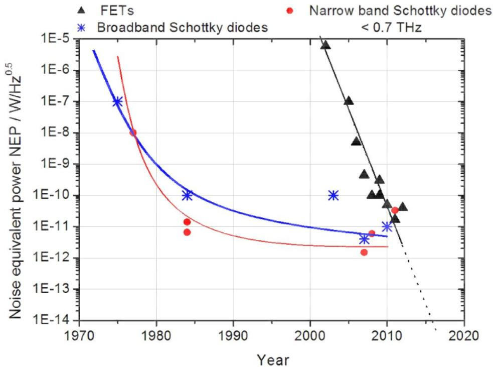
*Fig. 1: Direct detection NEPs of Schottky diodes and FETs at room temperature, extracted from the literature.*
